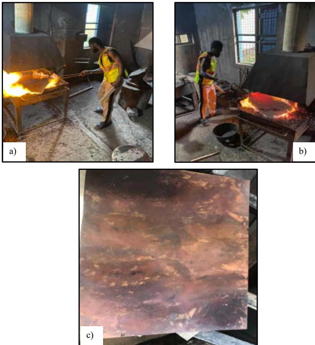
Figure 10: (a), Annealing of Copper Sheet, (b) metal sheet reaching red hot stage (c) Annealed Copper Sheet (Fieldwork, 2024).
