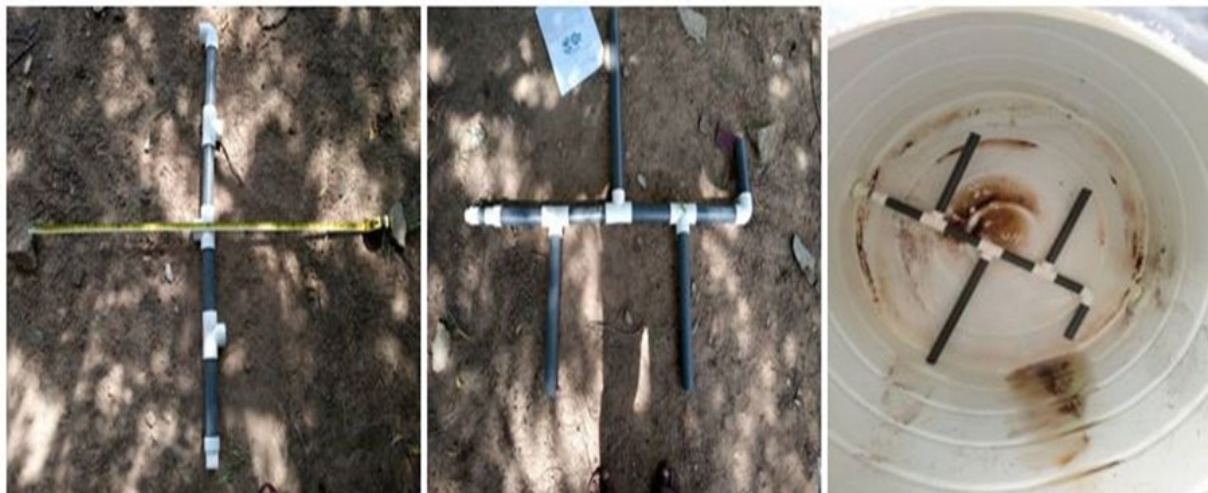
Figure 3: PVC Pipe Distribution Network System
